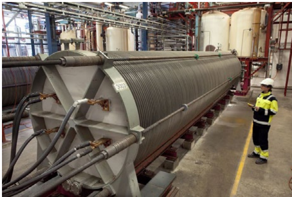
Figure 2: Nel-Akzo Nobel alkaline water electrolysis
